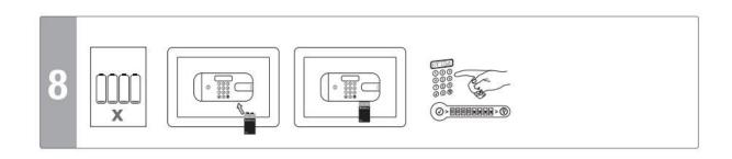
8. If the internal batteries are completely dead Please make sure to use a high quality 9V battery.
